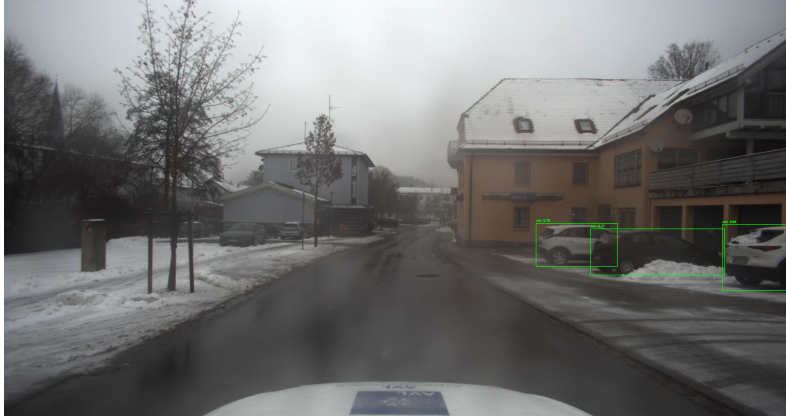
(a) OD confidence on the two leftmost bounding boxes is 0.78 and 0.77
