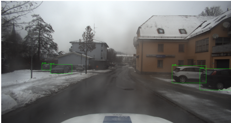
(b) OD confidence on the two leftmost bounding boxes is 0.85 and 0.87
