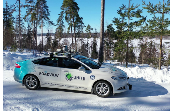
Fig. 1: The data gathering vehicle used evaluating DRLs in this paper. The driven journey is summarised in Section V-A. Photo credit: The Finnish Geospatial Research Institute FGI.
