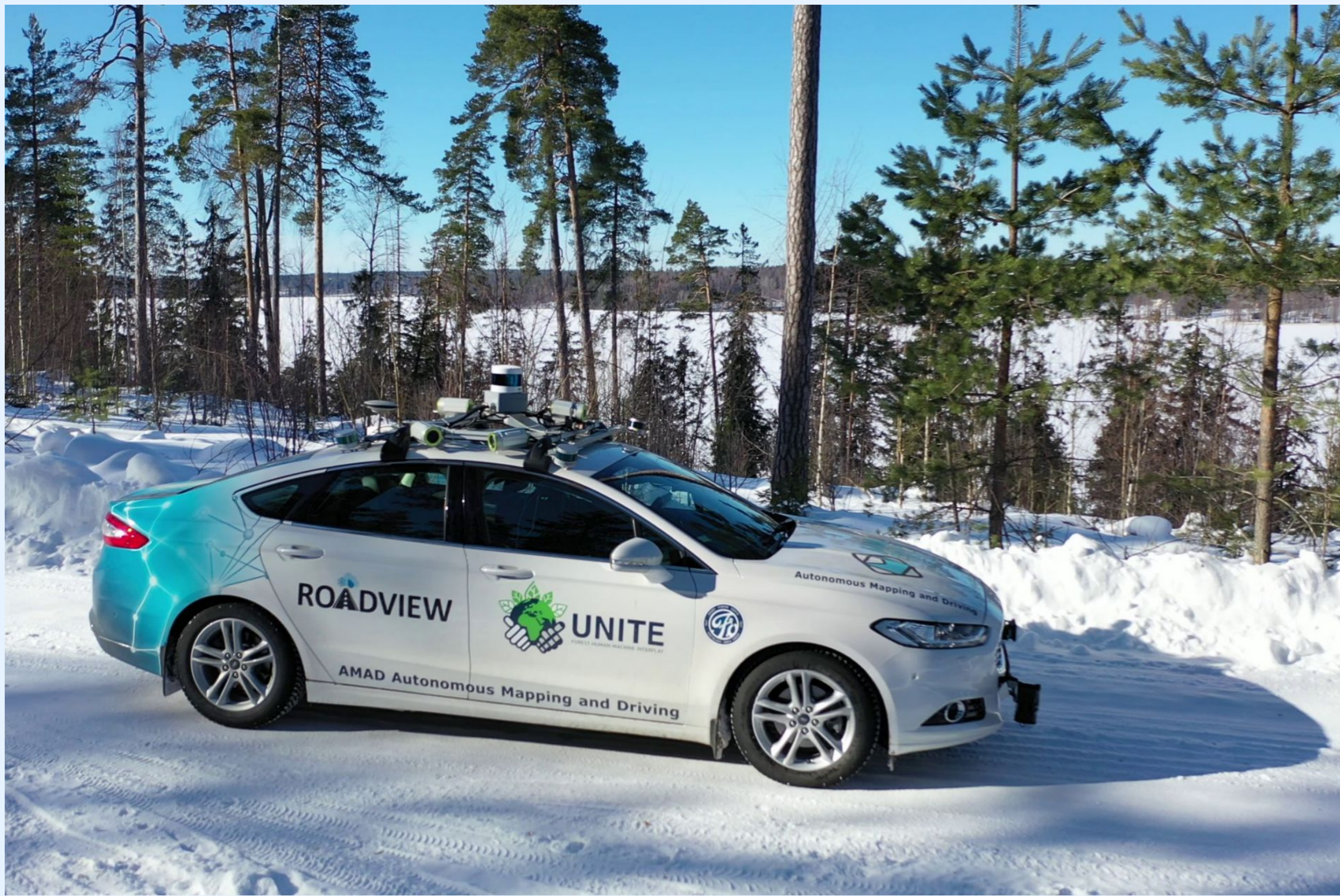
The data gathering vehicle used evaluating DRLs in this poster. Photo credit: The Finnish Geospatial Research Institute FGI.
